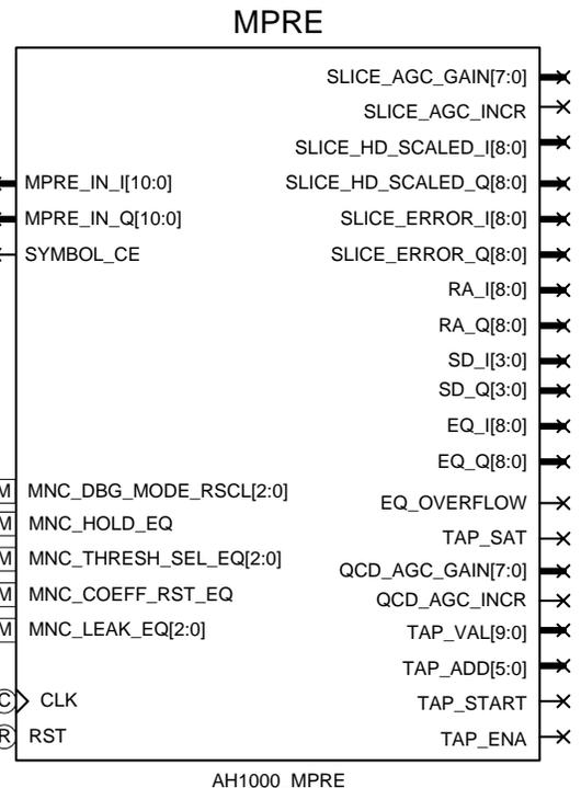
Figure 1. MPRE Schematic Symbol
