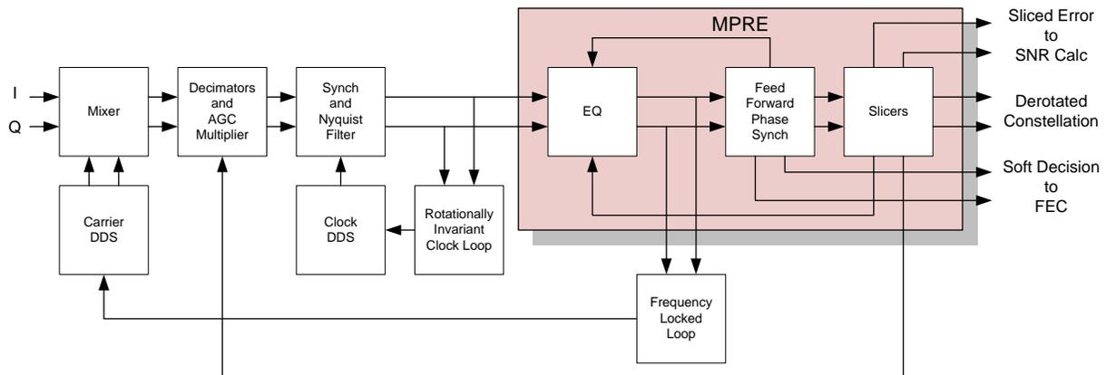
Figure 2. Signal flow diagram showing how the MPRE integrates easily into a typical demodulator.
