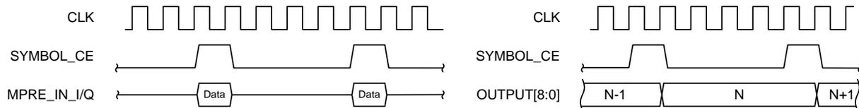
**Figure 6. Timing diagrams for the signal input path (left) and output paths (right).**
