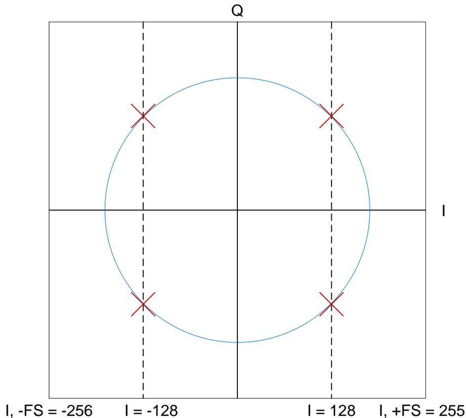
**Figure 5.** The AGC detectors seek to maintain the phase-locked received symbols on the red Xs. If the Equalizer output is within the blue circle the QCD\_AGC\_INCR signal is asserted to increase gain, and otherwise cleared to decrease gain. If the phase-locked RA\_I output is between the dashed lines, SLICE\_AGC\_INCR is asserted to increase gain and otherwise cleared to decrease gain. The Full Scale (FS) values shown are relative to the 9-bit output signals.
