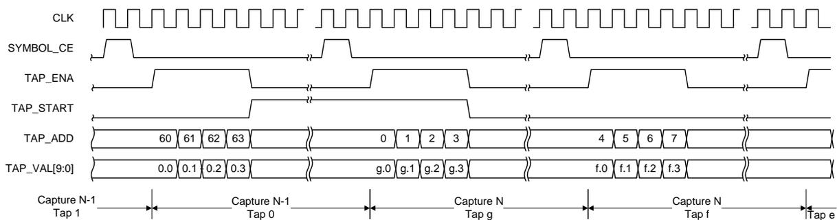
**Figure 4. Timing Diagram for the Equalizer Tap Coefficient Readout. The end of the N-1th coefficient capture and beginning of the the Nth capture are shown.**
