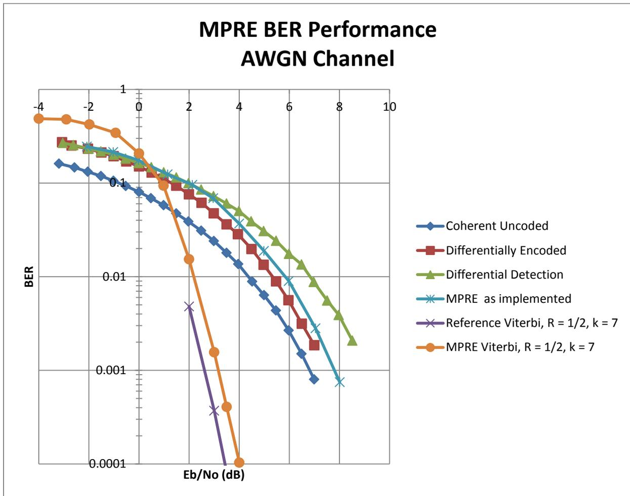
Figure 3. BER Performance of the MPRE in AWGN for both coded and uncoded cases. The MPRE generally operates within less than 1dB of a differentially-encoded coherent system.
