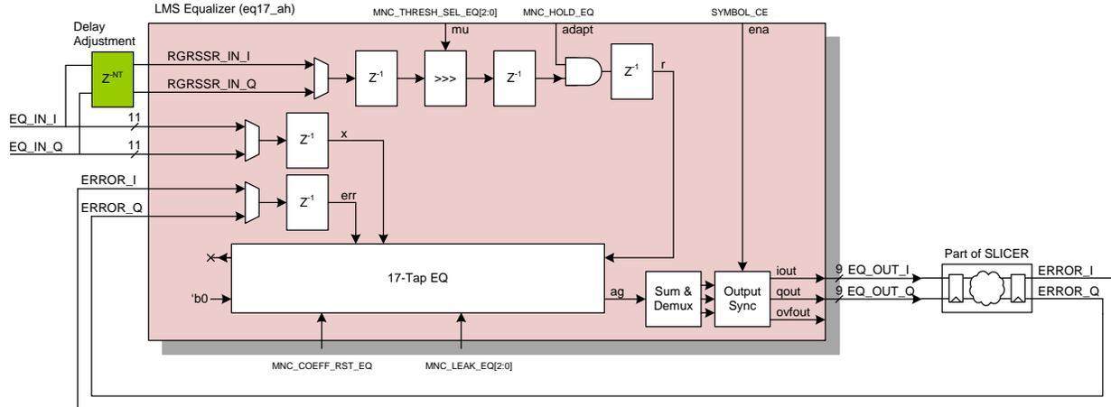
**Figure 2. LMS Equalizer block diagram showing integration with a constellation slicer and the Delay Adjustment block for synchronization of the Regressor and signed-Error signals.**
